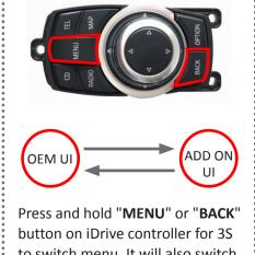
Press and hold "MENU" or "BACK" button on iDrive controller for 3S to switch menu. It will also switch to add on interface automatically after plugging a mobile phone or USB stick.
